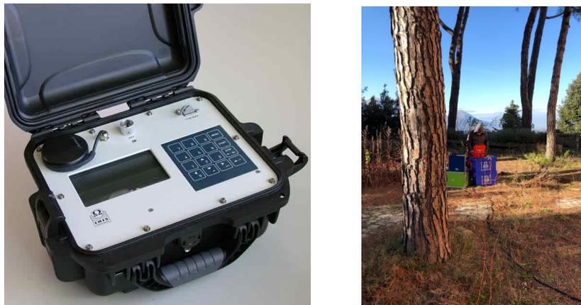
**Figure 74.** The Fullwaver equipment: example of receiver (left) and of an injection station.
