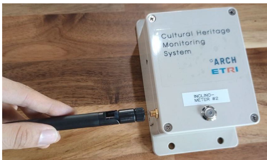
Figure 50. Installation of an external antenna
