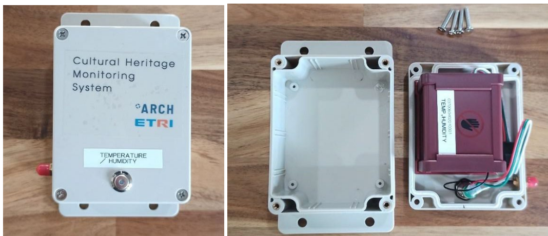
Figure 32. Temperature & humidity and vibration sensor node enclosure
