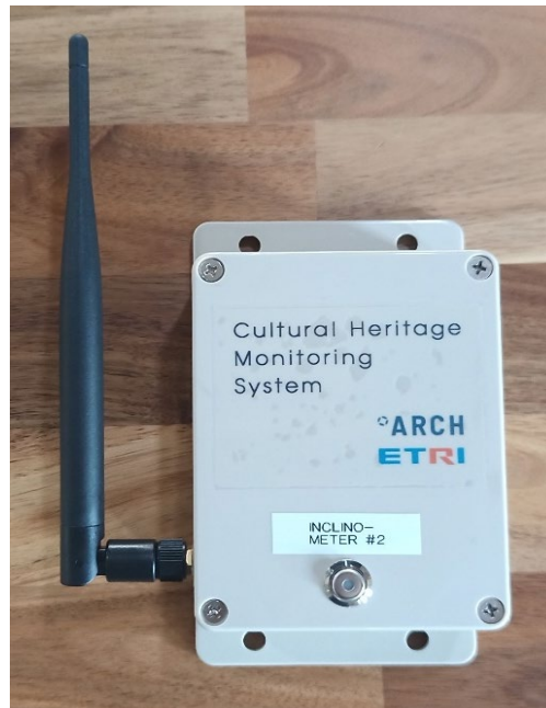
Figure 51. An example of proper antenna angle
