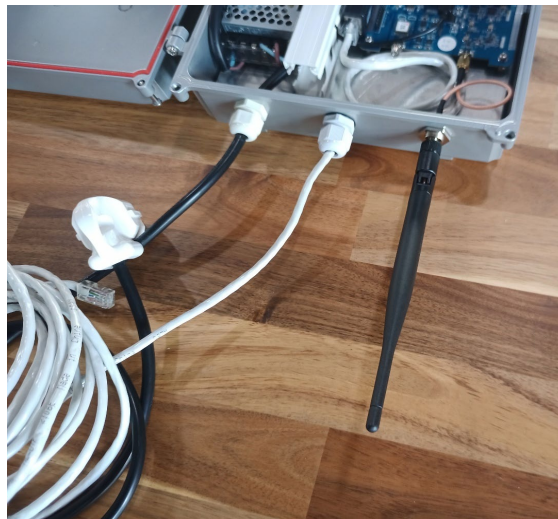
Figure 59. Antenna terminal on the bottom (antenna plugged in)
