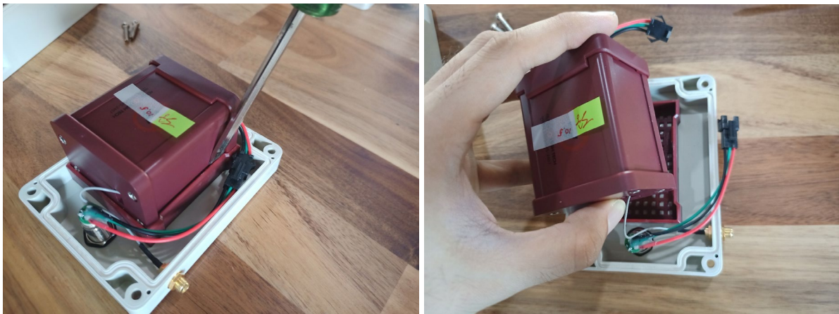
Figure 46. Separation of the inner box and outer box with a flat-head screwdriver
