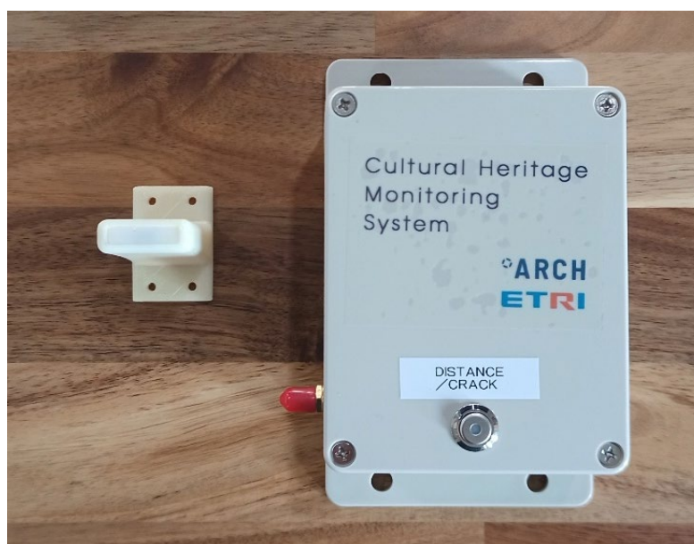
Figure 39. Crack sensor node with a magnet
