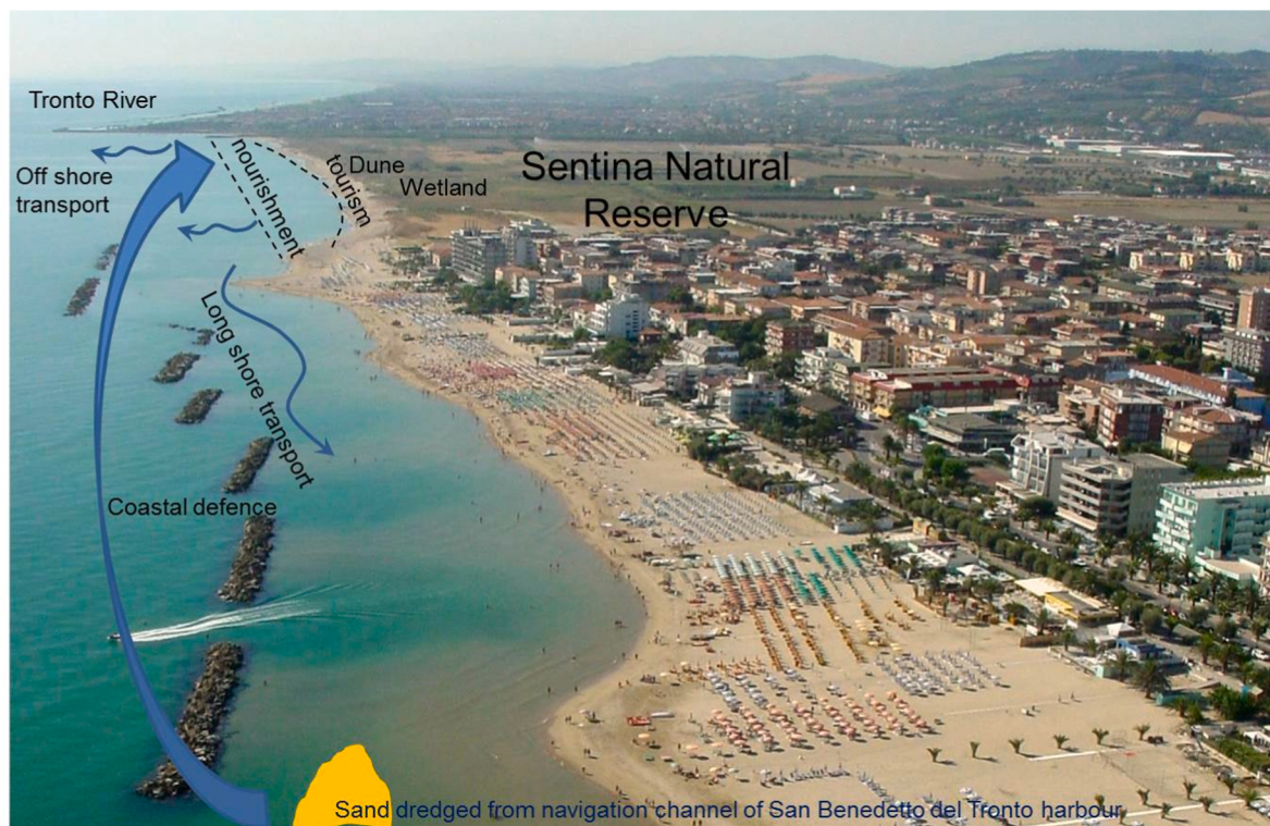
Fig. 10. Management scheme showing a summary of the sediment transport path implemented for the Natural Reserve of Sentina (background picture).
