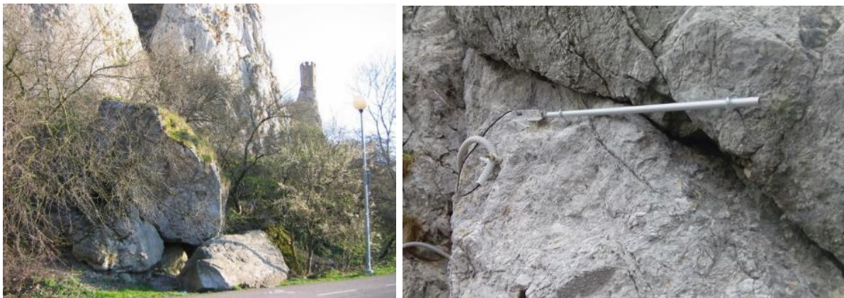
Figures 2.20 and 2.21. The danger of rockfall on the north-western side of the cliff (left), crack-gauge for monitoring rock displacement adapted specially for this Devin site using silica rods inert to temperature fluctuation (right). Photo: Bratislava City Museum, 2017.
