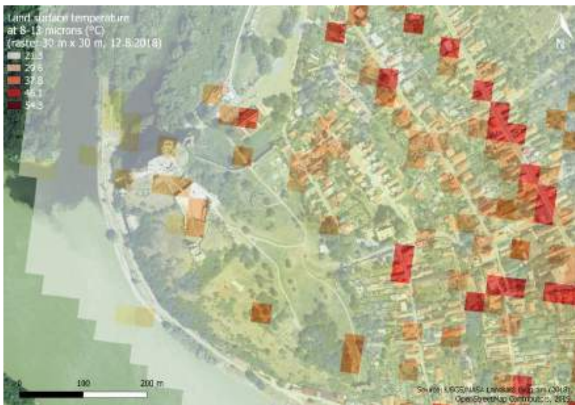
Figure 2.22. The land surface temperature model based on the evaluation of a multispectral satellite image of Landsat 8 [7]. The image shows the Devín Castle on the hill on the left.
