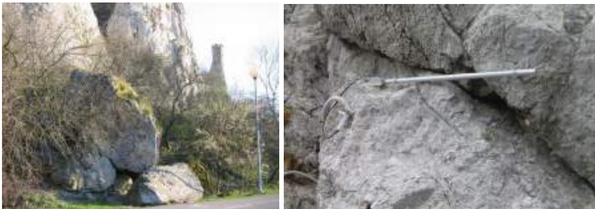
Figures 2.20 and 2.21. The danger of rockfall on the north-western side of the cliff (left), crack-gauge for monitoring rock displacement adapted specially for this Devín site using silica rods inert to temperature fluctuation (right). Photo: Bratislava City Museum, 2017.
