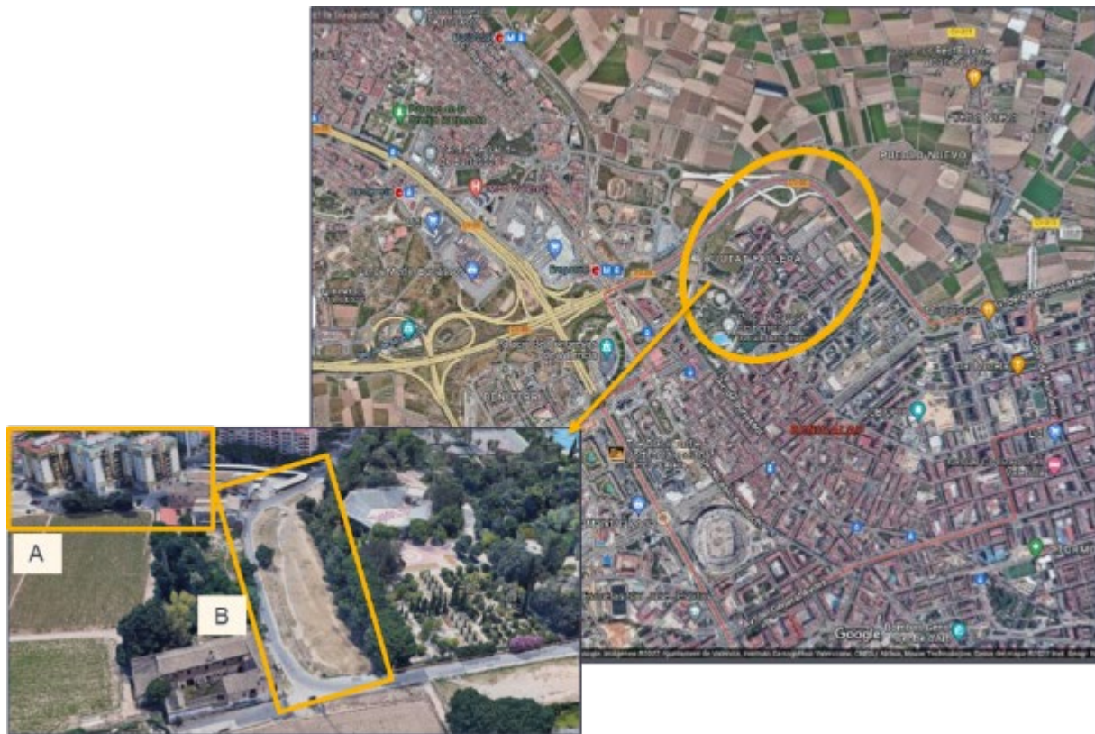
Figure 56. Modelled areas. A: Green roofs, green façade, extra trees and grass (as garden) were modelled in a street. B: Urban forest, grass as green permeable pavement, urban vegetable garden, pergola as shading, fountain, pond, water spraying as playground
